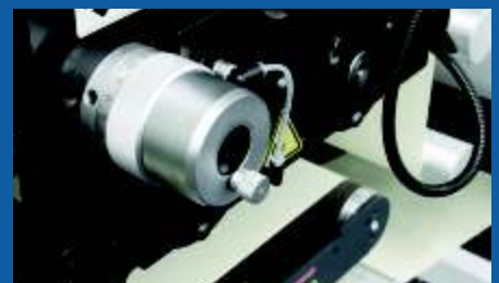
Gap control system GapMaster
