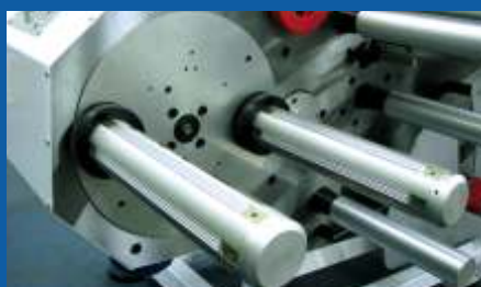
Semi-turret version of rewinders with the option of simultaneous wound on two spindles
